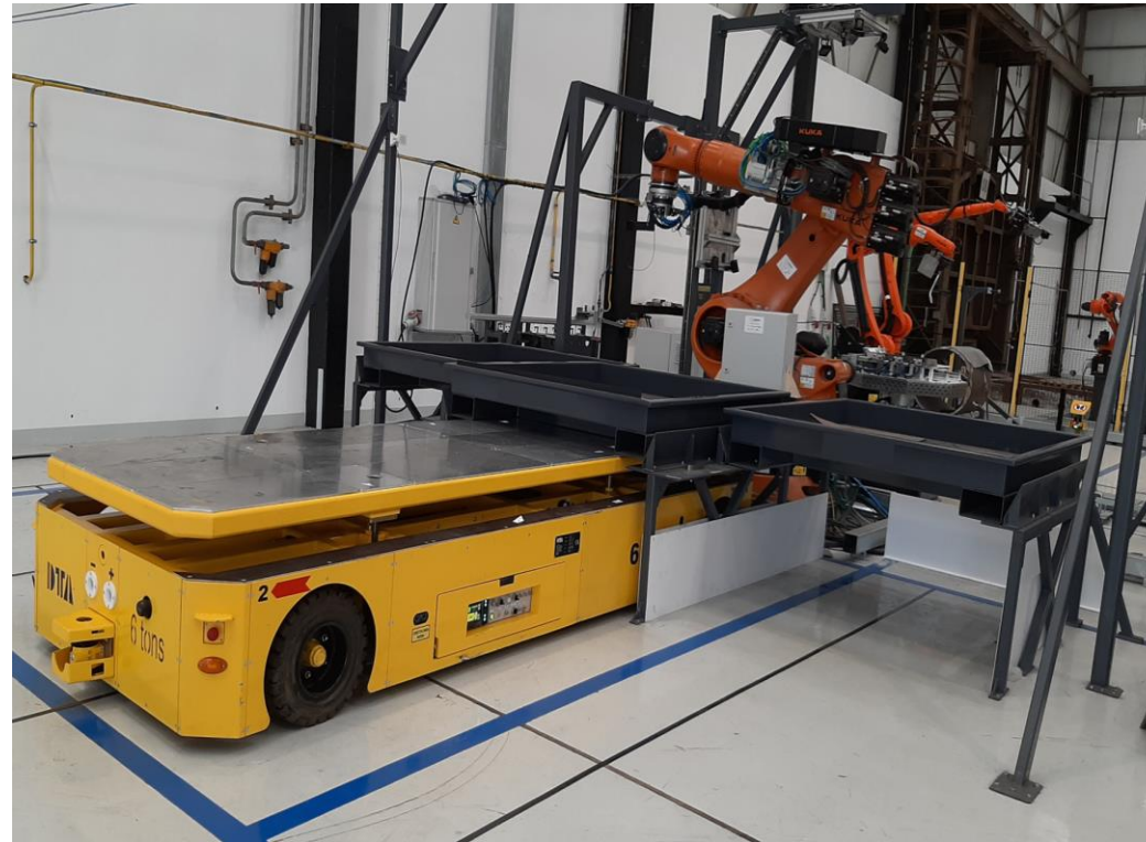
Transfer of materials into the welding cell
