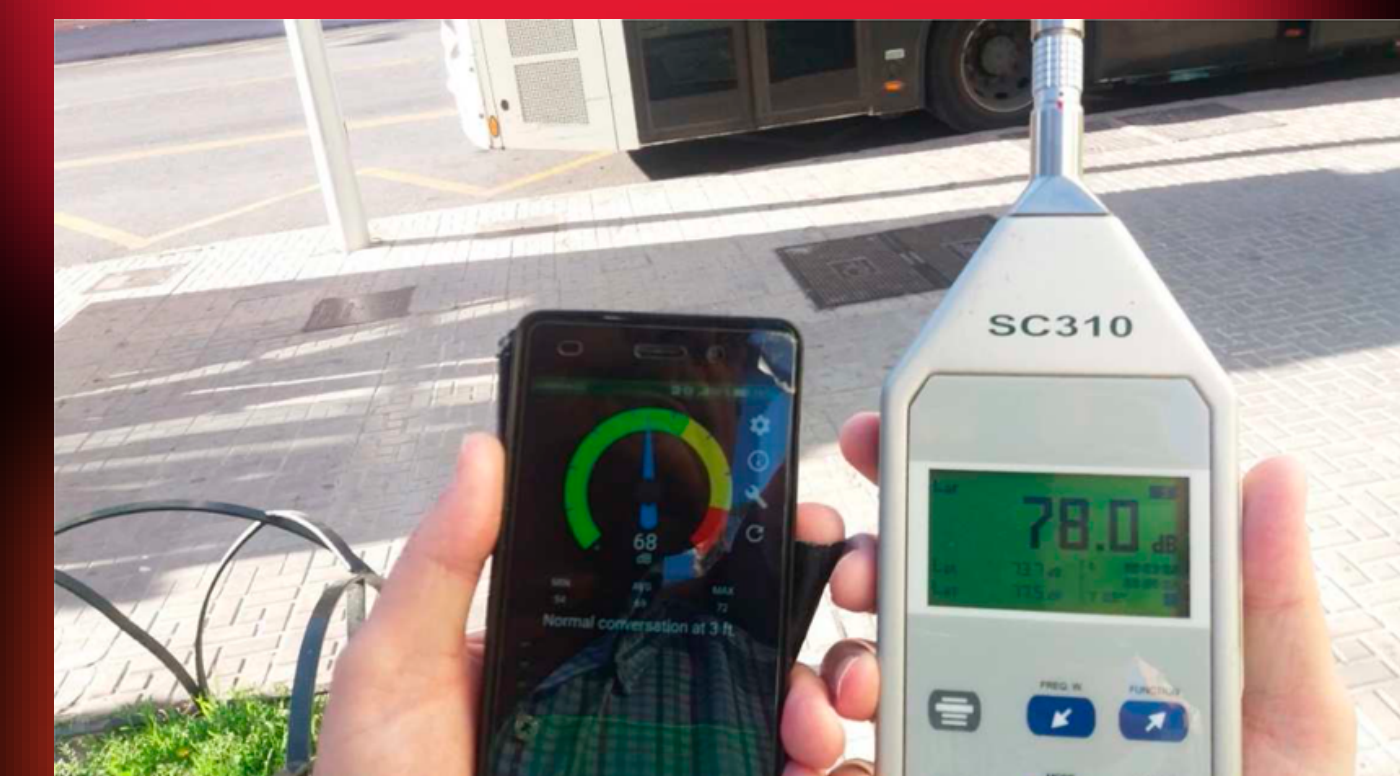
Image 2: Comparison of values recorded with the sound level meter and mobile phone at location 6 of Cristo de Mena School.
