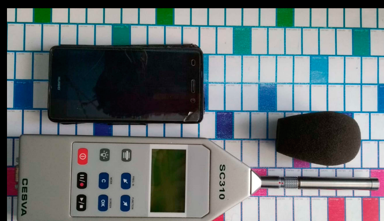
Image 1: Measurement equipment used in measurements. Above is a Samsung Galaxy brand mobile, equipped with the Sound Detector and Sound Meter apps. Below, a type 1 sound level meter, CESVA brand.
